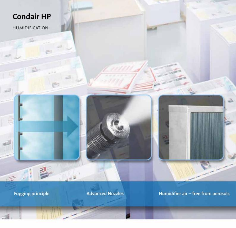
The Condair HP supplies demineralized water 70 bars of pressure to atomizer nozzles installed inside of an air duct. Advanced atomizing nozzles generate an extremely fine mist which is rapidly absorbed into the airstream while a highly efficient droplet separator contains any excess water within section. Cool, humidifier air is then released into rooms, creating a healthy environment and enhancing productivity.
